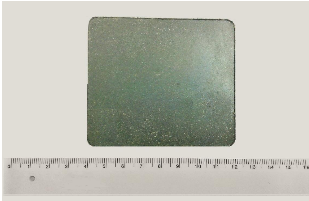
Figure 4.2. Produced preceramic matrix composite sample by warm pressing technique.
