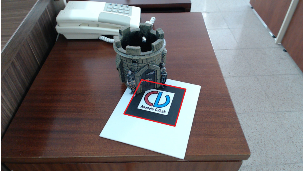
Figure 4.13: A marker whose one corner is occluded. Since unoccluded vertices and corners are on a single edge segment, this marker will be detected.
