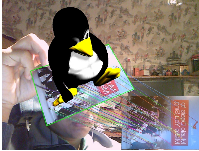
Figure 1.1: A depiction of markerless AR [1]. Lines represent correspondences between features detected by FAST [2].
