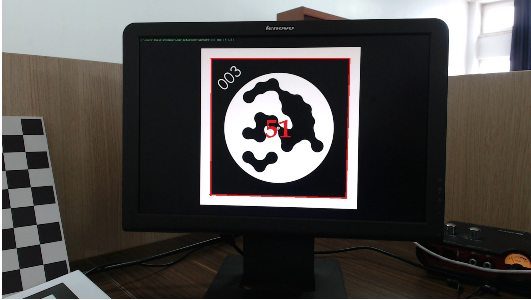
Figure 3.2: Intermarker confusion example. Marker #3 falsely identified as marker #51. This image is for illustration purpose only, it is not a result of the EDMarkers detection algorithm.
