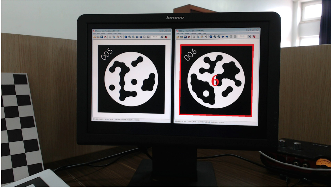
Figure 3.3: False negative example. Marker #5 is not detected even though it is present. This image is for illustration purpose only, it is not a result of the EDMarkers detection algorithm.
