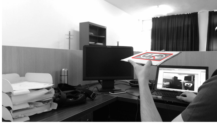
(d) The marker is seen at an extreme angle and there is blooming due to excessive lighting.
