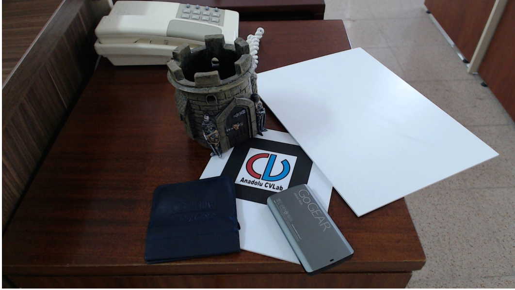
Figure 4.12: A marker whose all corners are occluded. Since the occlusions will break the edge segments, extracted line segments will belong to different edge segments.
