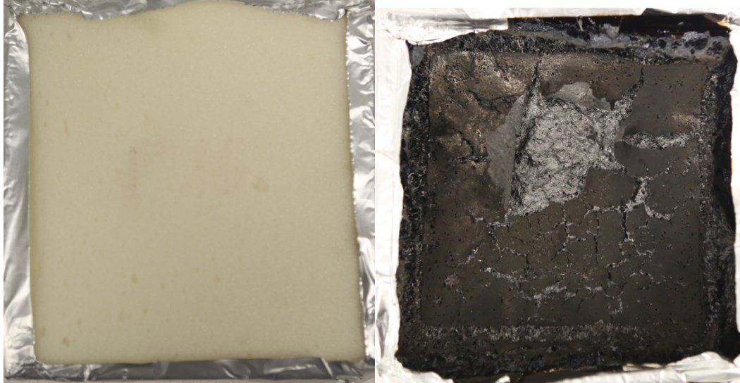
Figure 4.3. RPUF sample for cone calorimeter test (before and after burning)
