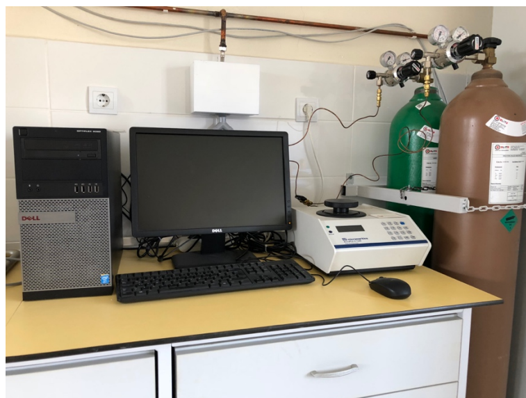
Figure 3.3. Gas displacement pycnometer system
