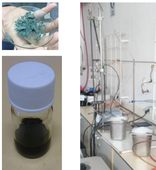
Figure A.21. Dried biomass (left top), produced bio-oil (left down) and fast pyrolysis set up (right)
