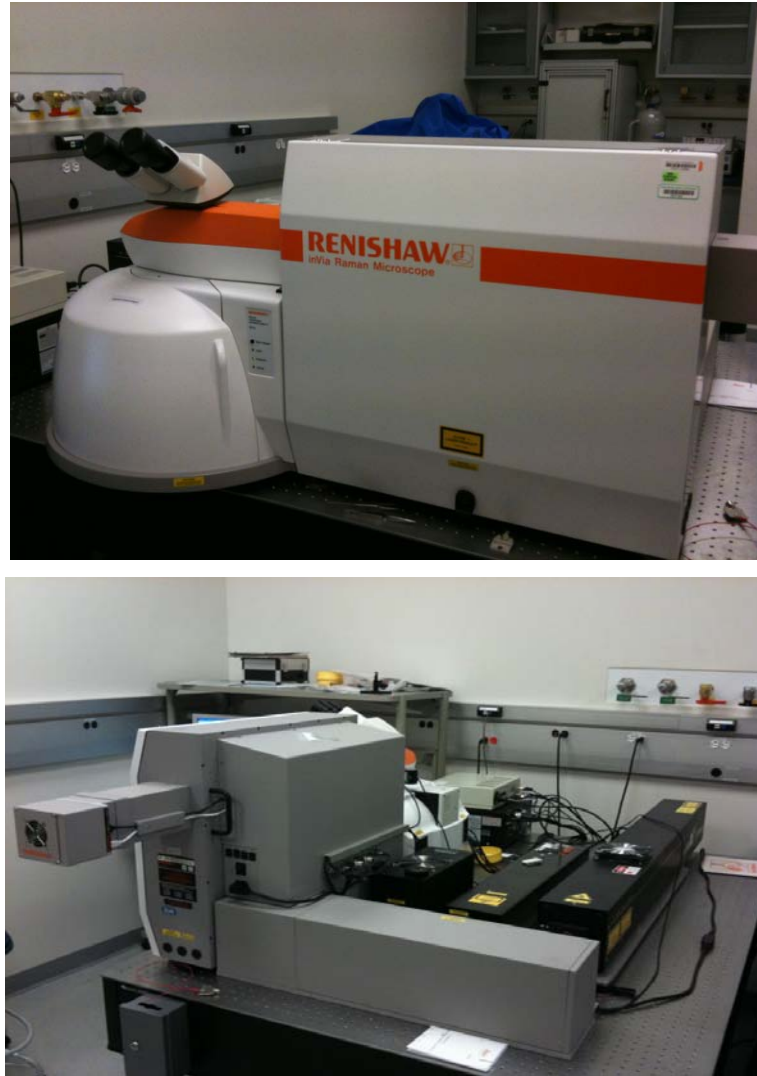
Figure 4.4. Renishaw inVia Reflex Micro-Raman Spectrograph used in the experiments.
