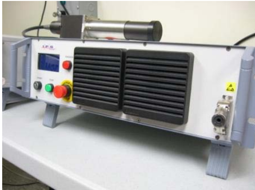
Figure 10.2. High power IPG laser system (1070 nm, 100 W).
