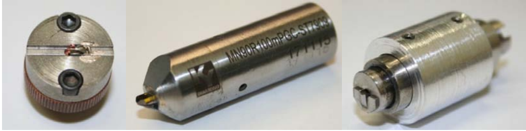
Figure 10.1. Various types of diamond tools will be used in \mu -LAM.
