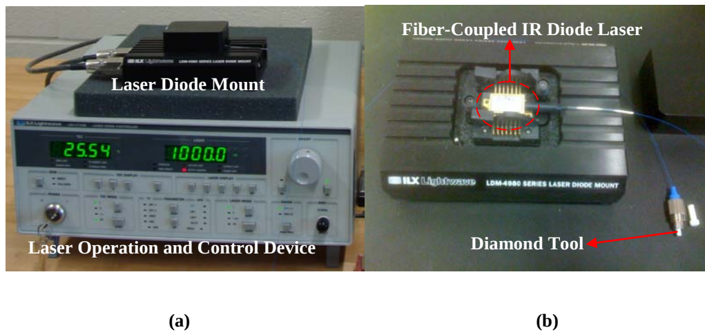
Figure 4.2. The laser heating system used in the experiments.
