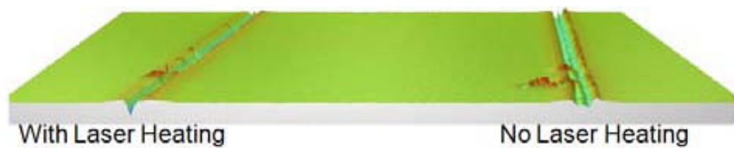
Figure 9.7. 3D scratch profiles of the Si scratches with and without laser heating (related to the same area imaged in Figure 9.6).
