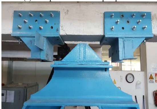
(c) Close view after mounting of U-shaped plates
