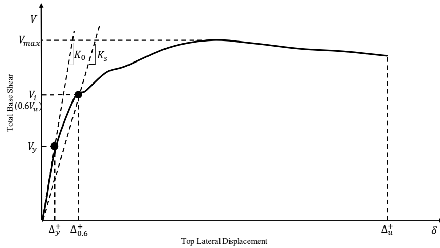
Figure 5.3. Definition of structural stiffnesses
