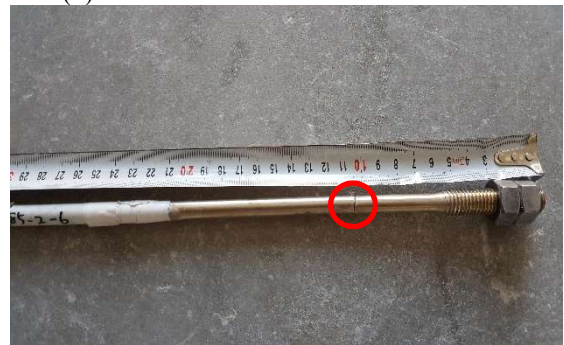
(f) View of CuAlMn-2 after the test
