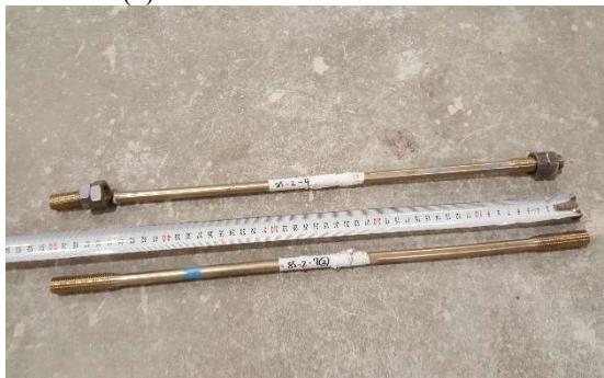
(e) View of CuAlMn 3&4 after the test
