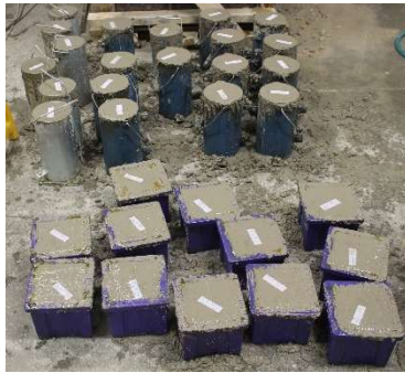
(a) Cylindrical and cubic specimens after casting
