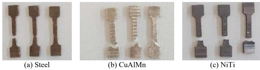
Figure 3.13. Tested dog-bone shaped specimens of upgrading materials
