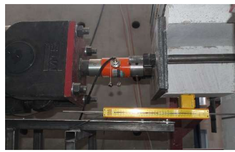
(b) Close view of MTS-frame connection
