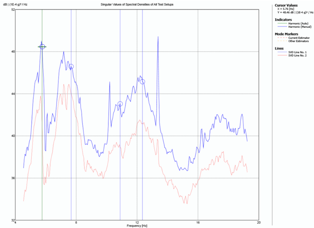
Figure 4.4. Singular values of spectral densities of all setups, EFDD method
