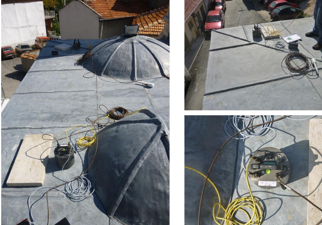
Figure 4.3. Test equipment; Left: Base station and 1st station, Right top: 4th station, Right bottom: accelerometer at the base station
