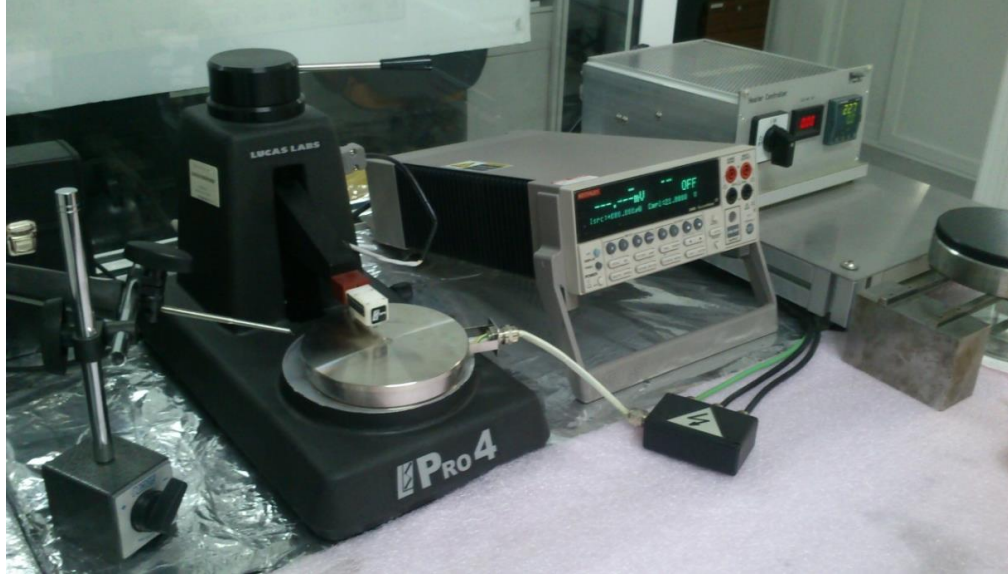
Visual 2.2. FPP system present at Advanced Technology Thin Film Laboratory of Anadolu University
