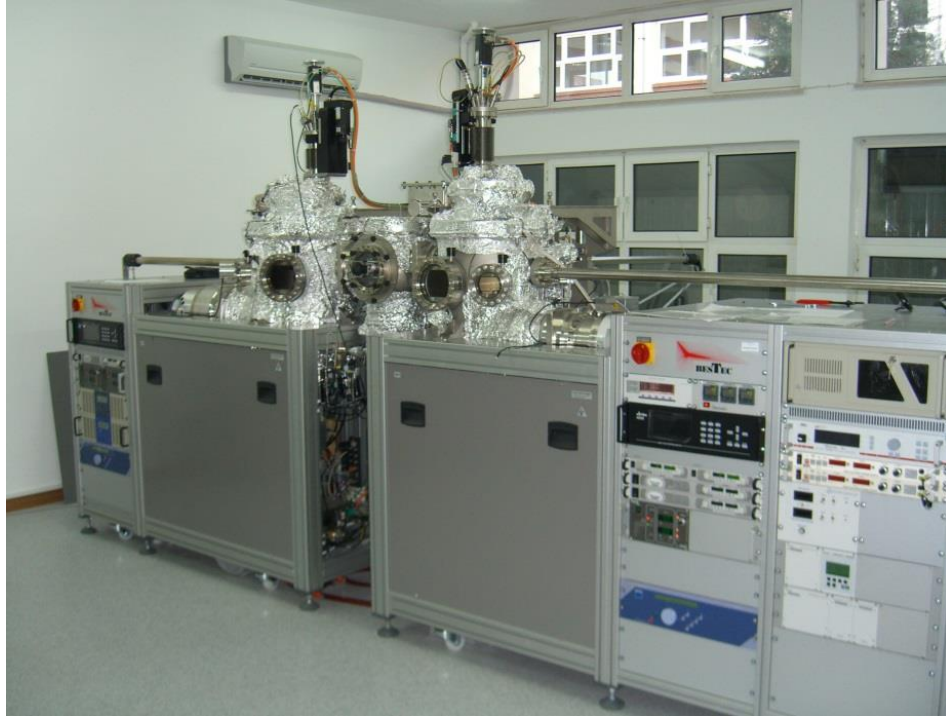
Visual 2.1. Bestec Ultra High Vacuum Sputter System present at Advanced Technology Thin Film Laboratory of Anadolu University
