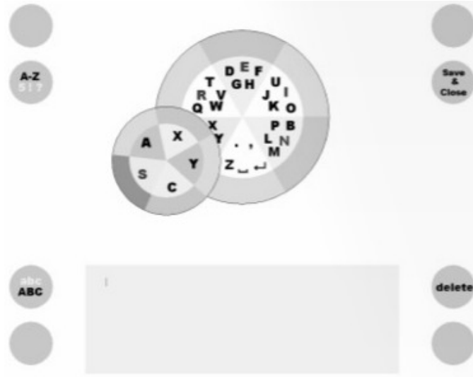
Figure 4.6: pEYWrite’s user interface. The circular pies in the middle are used to enter letters, which appear inside the textbox at the bottom. Other buttons shown on the sides provide auxiliary functionality.
