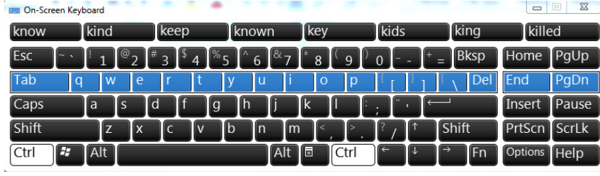
Figure 4.1: Scanning keyboard in Windows 7. The current scan is at row 3. Letter ‘k’ has been selected in the previous scan; therefore, the keyboard displays word suggestions at the first row.
