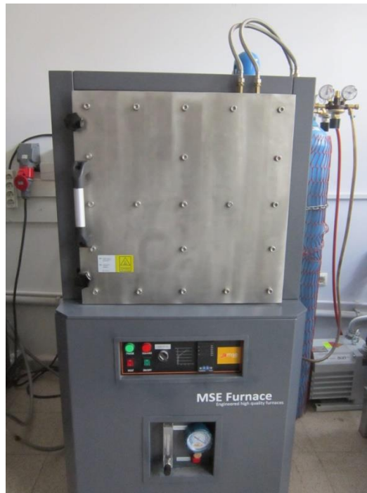
Figure 5.5. The furnace used in hot rolling, homogenization and annealing processes.
