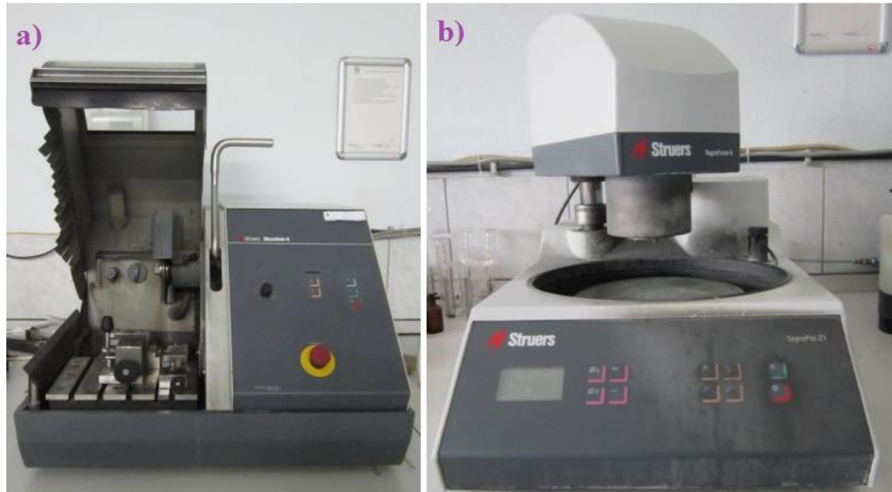
Figure 5.8. a) Struers Discotom-5 cutting device and, b) Struers TegraPol-21 polishing device.
