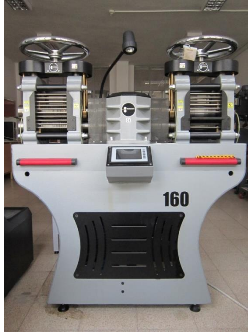
Figure 5.6. Durston (DRM160) machine used for rolling processes.
