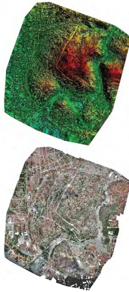
Figure 1: Orthomosaic and the corresponding sparse Digital Surface Model (DSM) before densification.
