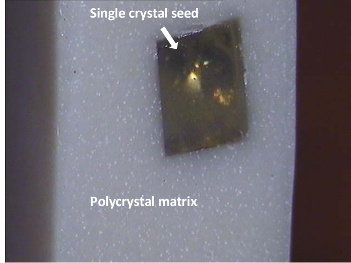
Figure 9.11. Stereo microscope image of single crystal seed material embedded in polycrystal matrix
