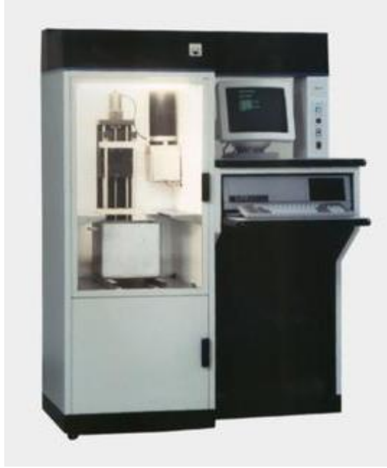
Görsel 2.3. 3D Systems řirketinin ürettiđi ilk steryolitografi yazıcı, 1987 Kaynak : https://www.3dsystems.com/our-story
