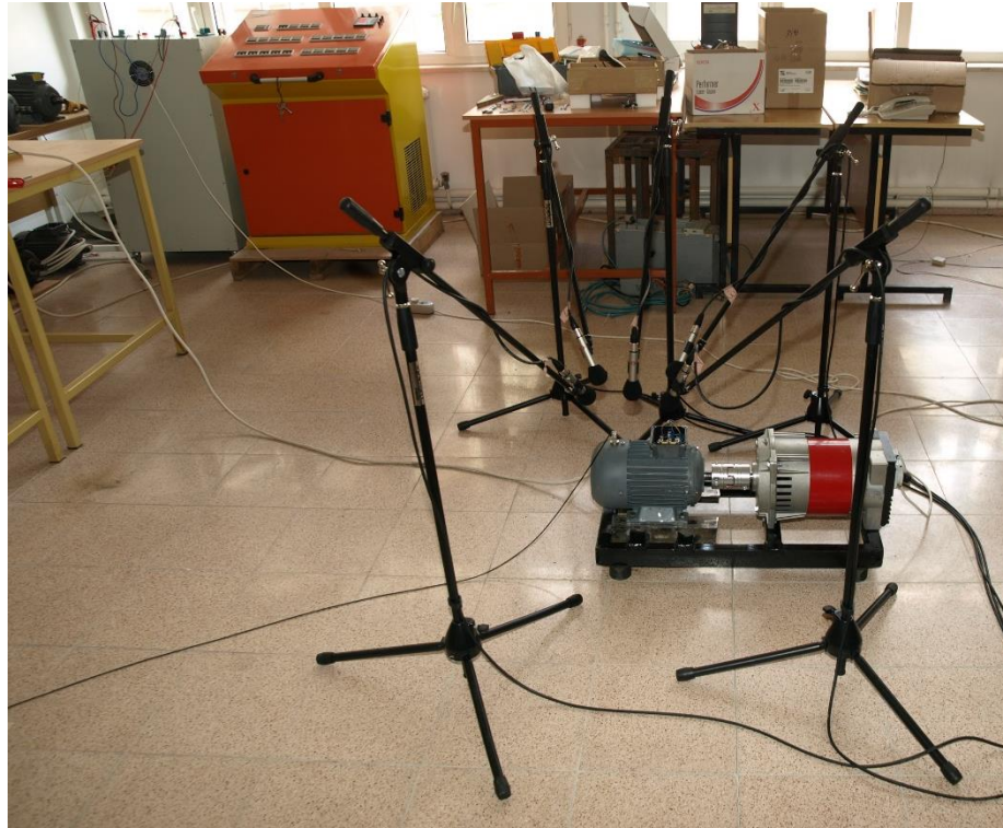
Figure 2.6. Experimental Setup for vibration and acoustic data
